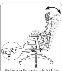
Life the handle upwards to lock the tilt or downwards for free-floating action.
