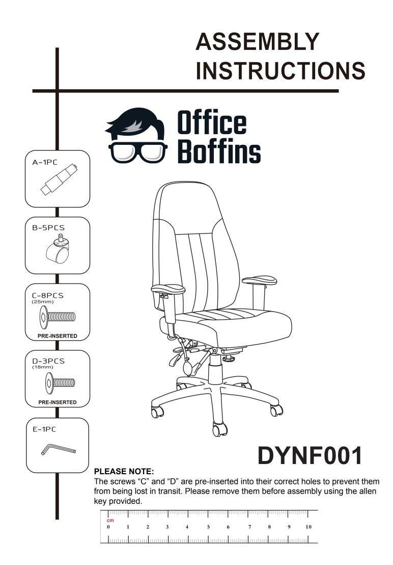
Do not tighten bolts fully until you have completed assembly. DO NOT USE A POWER DRILL TO TIGHTEN THE SCREWS. TIGHTEN BY HAND WITH THE ALLEN KEY PROVIDED.
