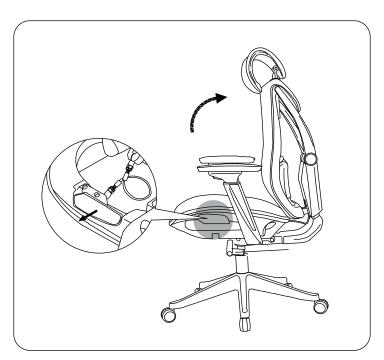
2 Position Back Angle Tilt, pull the lever out to release the back angle tilt. Pull out once and lean back into the 1<sup>st</sup> position. Pull out again to lean back into the 2nd position.
