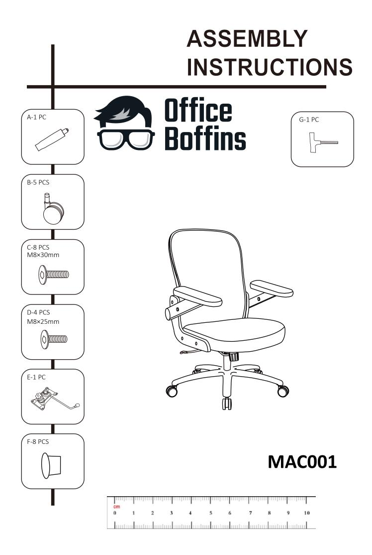
Do not tighten bolts fully until you have completed assembly. DO NOT USE A POWER DRILL TO TIGHTEN THE SCREWS. TIGHTEN BY HAND WITH THE ALLEN KEY PROVIDED.
